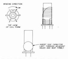
fig. 3. Coil winding and lead identification.
